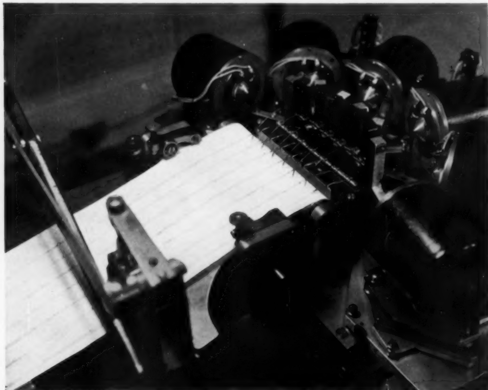
FIG. 3. Enlarged view of electromagnets and 13 pens which write on paper. The flying shears are clearly shown.
